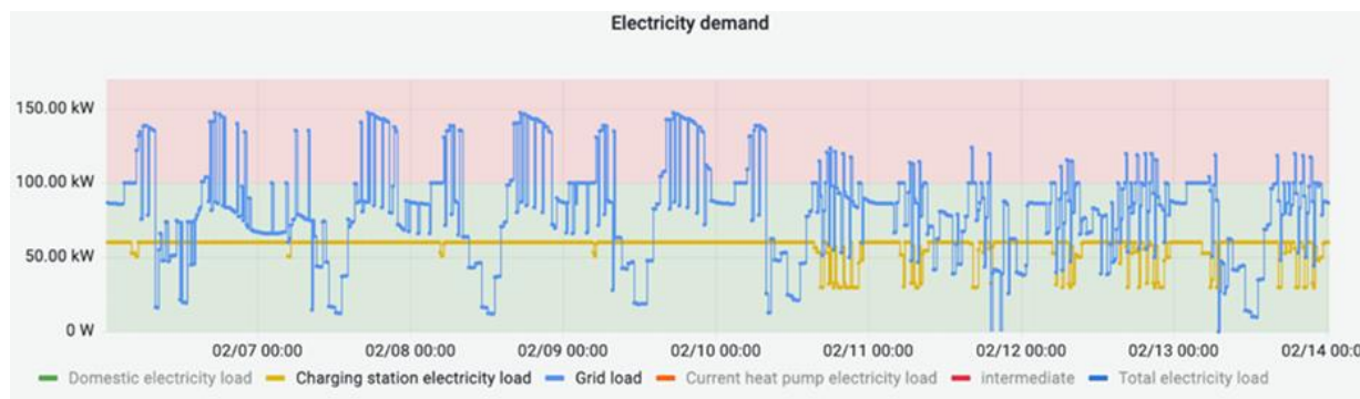
Figure 13: Example of Peak Shaving above 100kW Threshold on the Collective Load Curve (DuCoop EAN)
